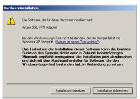
The installation wizard will copy the necessary files on your system. A virtual network card will be installed during the installation process. Since the relevant driver is not certified by Microsoft, a corresponding caution message will appear during the installation process. You can ignore this message.
